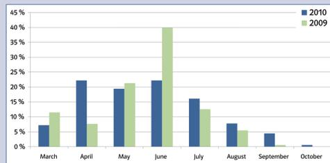
Fig. 1: Relative occurrence of the maximal feed in power of 150 distributed PV systems in Bavaria.
