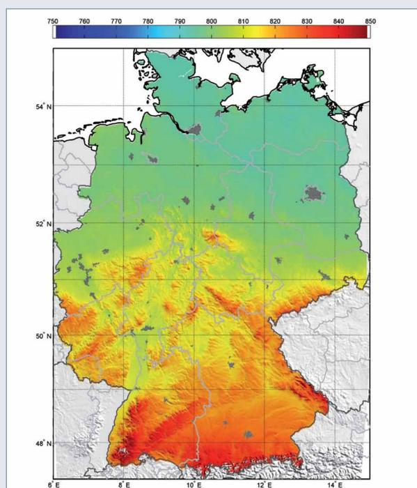
Fig. 3: Maximal feed in power of a typical south orientated PV system for Germany in  $\text{W per kW}_p$  installed STC power.
