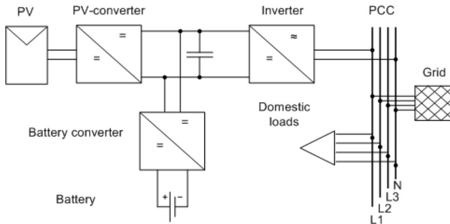
Fig.5: Sol-ion system layout (Büdenbender et al., 2010)
