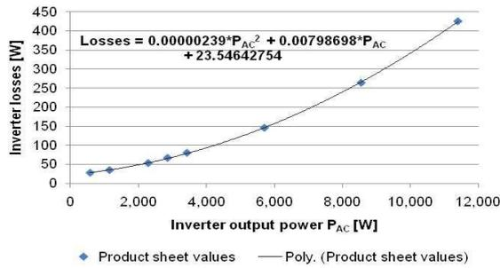
**Figure 4: Inverter losses characteristic and the derived polynomial function.**
