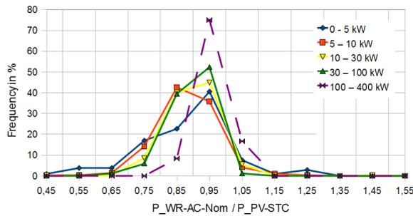
Figure 2: Frequency distribution of current inverter sizing in South-East Bavaria.
