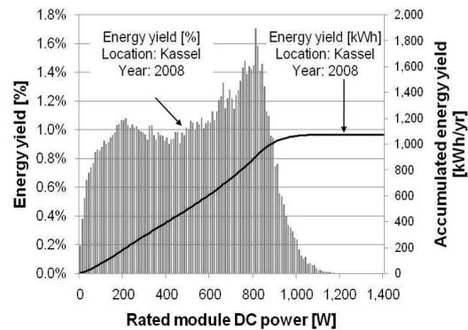
Figure 3: Energy yield of the used DC power measurement data with a timely resolution of 1 minute.
