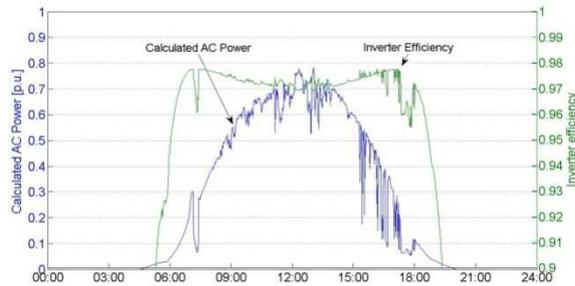
**Figure 5: AC power feed-in as a result of the inverter model for a summer day in Kassel in 2008.**
